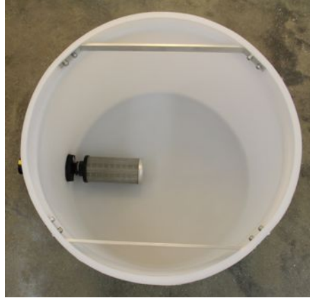
Figure 4. The downstream reservoir has aluminum struts.
