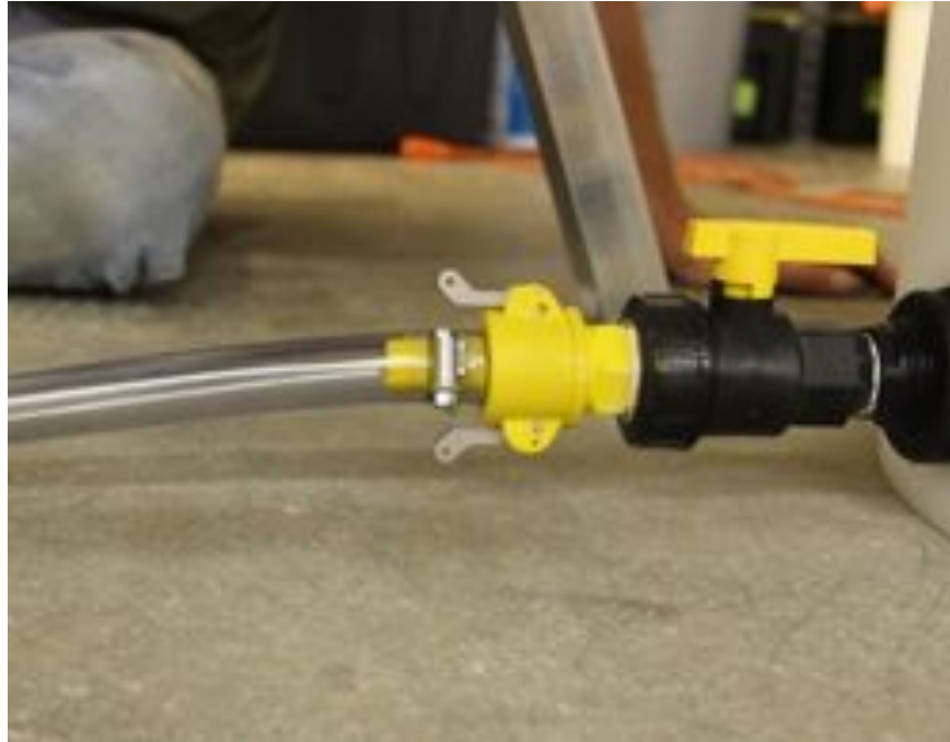
Figure 10. How the tubing fitting and reservoir valve look when properly connected. Note that the metal clips must be snapped down toward the tubing.
