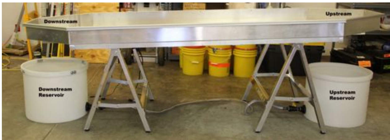
Figure 3. This is how the model should look after completing steps four and five. Note the orientation of the two reservoirs with respect to the upstream and downstream ends of the box.
