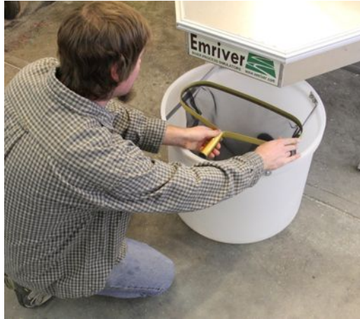
Figure 14. Place the sediment trap on the aluminum struts in the downstream reservoir.
