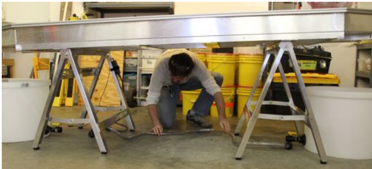
Figure 7. The one-inch tubing connects the two reservoirs.
